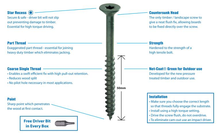
Timber-Tite® is a universal, heavy duty timber fixing that replaces cup square bolts and coachscrews for an easy, quick, secure and neater fix.
